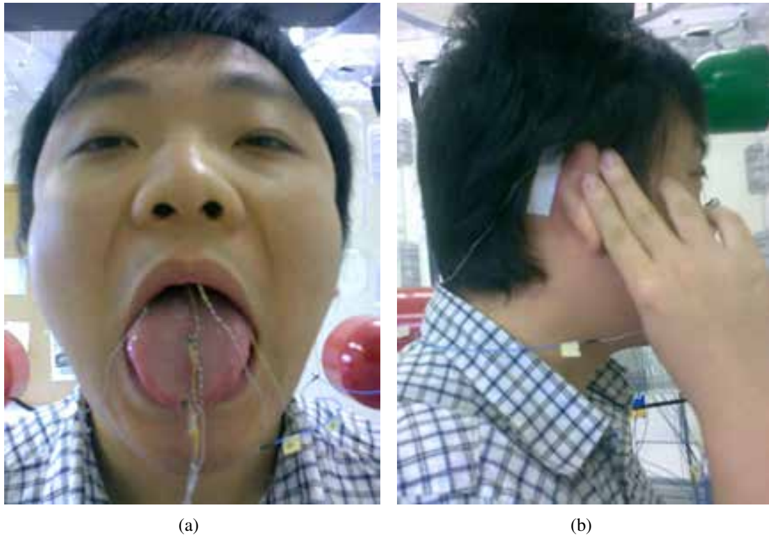
Figure 2.10: An example deployment of the Articulograph AG500 system motion sensor. In common practice, at least three sensors are used to identify the rotational movement of the head, or a mandible, as shown in Figure 2.10(b).
