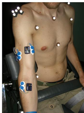
**Figure 8.3:** *The subject is positioned on the Biodex. Wireless EMG dipole electrodes are fixated on right arm of the subject. Furthermore, positioning markers are placed on his upper body.*
